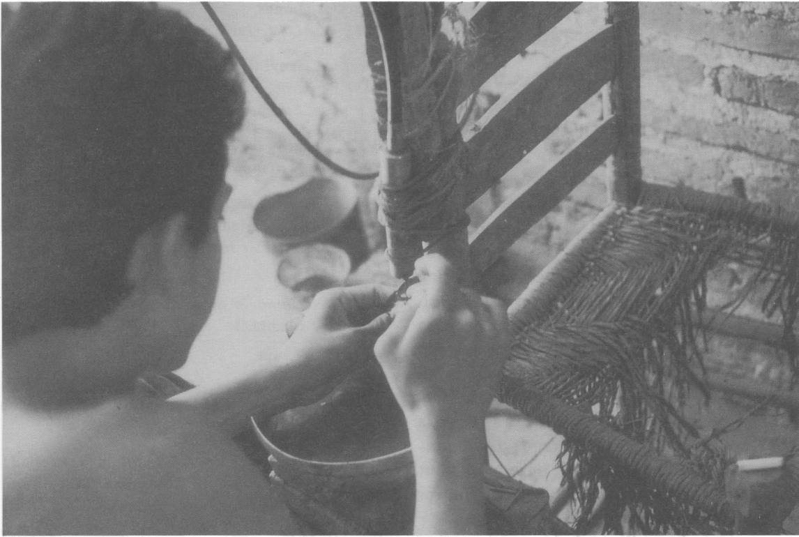
Figure 15. A young man drills a stone bead in Iguala, Mexico (1985). After the guild system was abolished following the 1910 Revolution, anyone who wanted to make a bead could. Those who chose to do so had to figure out how to do it. This bead is being drilled using a most unorthodox method involving a bent umbrella rib and commercial "emery" slurry.
